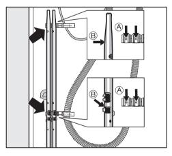
■ Fasten the shipping struts at the rear side of the washer. Take care to insert the drill holes, (B), into the clamps, (A).
